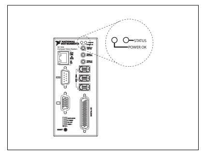
Figure 3-1. POWER OK and STATUS LEDs
